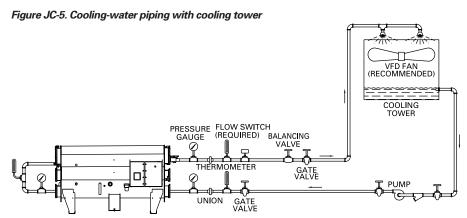
COOLING-TOWER PIPING WITH COOLING-WATER TEMPERATURE CONTROL
